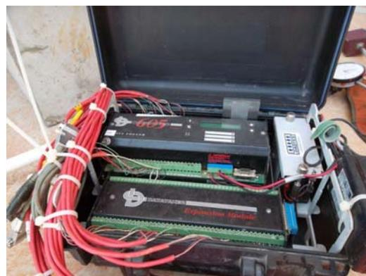
*Strain Gauge Leads Connected To Data Logger*
