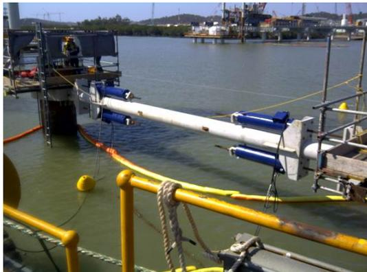
Arrangement of Lateral Loading Setup
