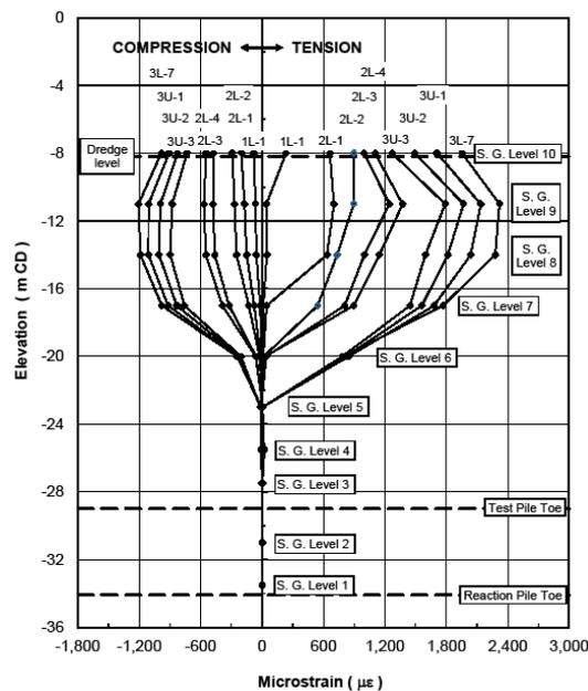
Typical Pile Shaft Strain Distribution
